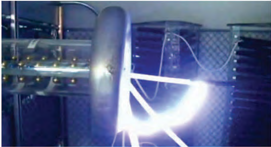
Figure 9. CUT#4. Photo of flashover. Positive polarity.
