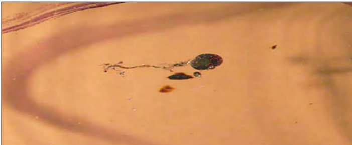
Figure 2: Magnified arcing area on the glass, showing a damaged tube wall.
