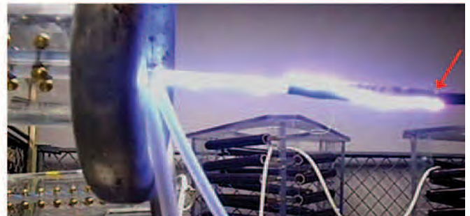
Figure 11. CUT#6. Photo of flashover. Positive polarity.
