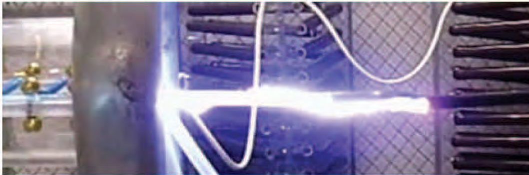
Figure 10. CUT#5. Photo of flashover. Positive polarity.
