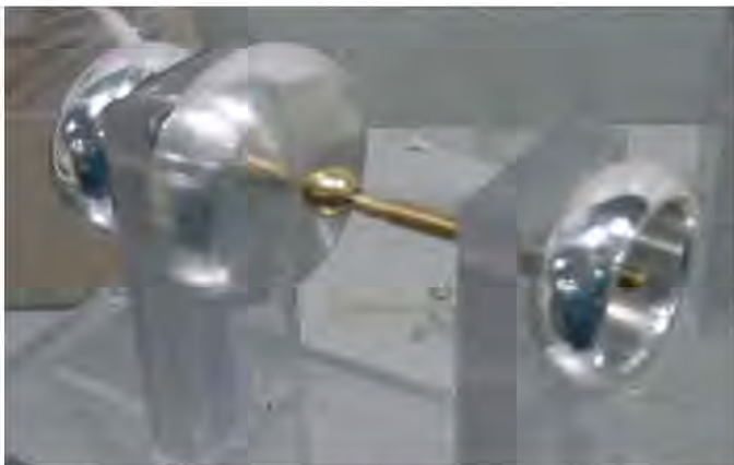
Figure 3. Sphere-to-plane spark gap.
