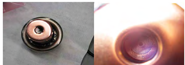
Figures 10, 11: Focal spot damage caused by inadequate anode cooling and thermo-mechanical stress
