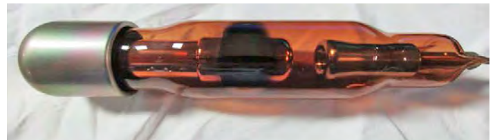
Figure 9: An X-ray tube operated in a hot oil environment with a thin layer of carbonized oil etched onto its surface.
